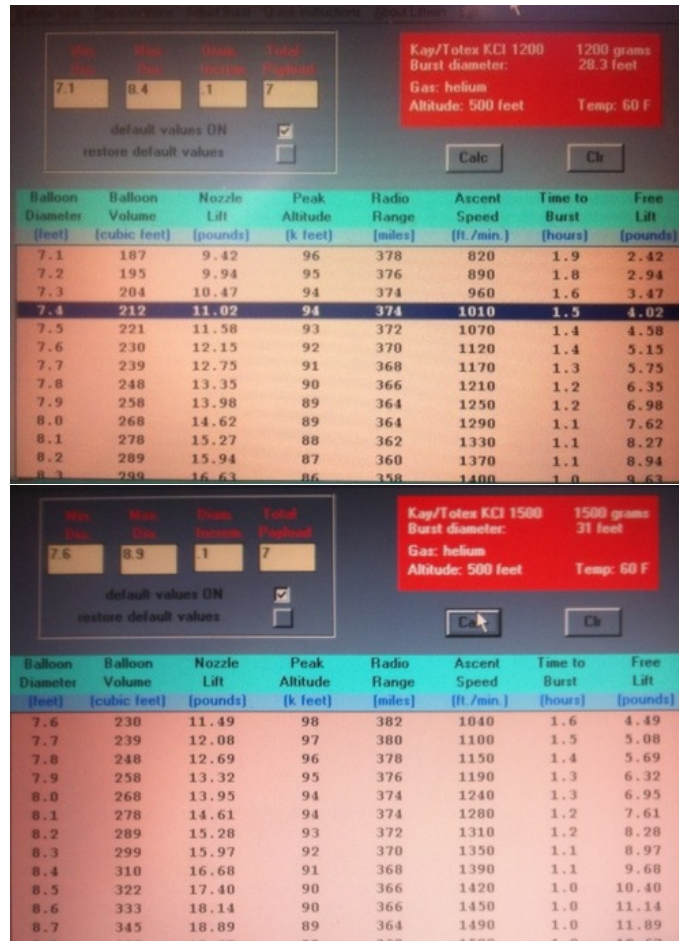
Figure 2: Balloon parameters for a (upper) 1200 gram balloon and (lower) 1500 gram balloon.
