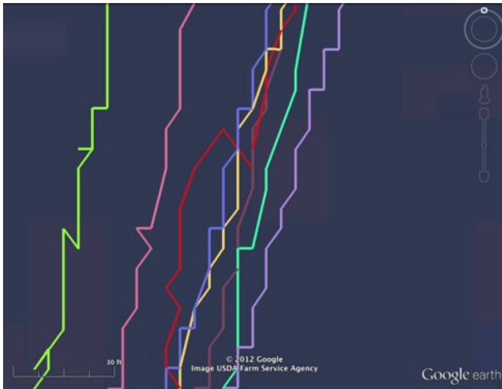
Figure 20: GPS jitter during Connecticut launch
