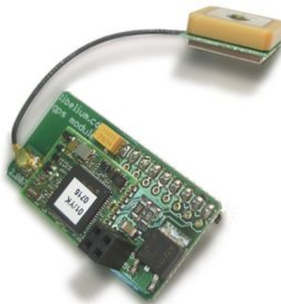
Figure 8: the GPS module used in the Duck payloads. Image from www.cooking-hacks.com
