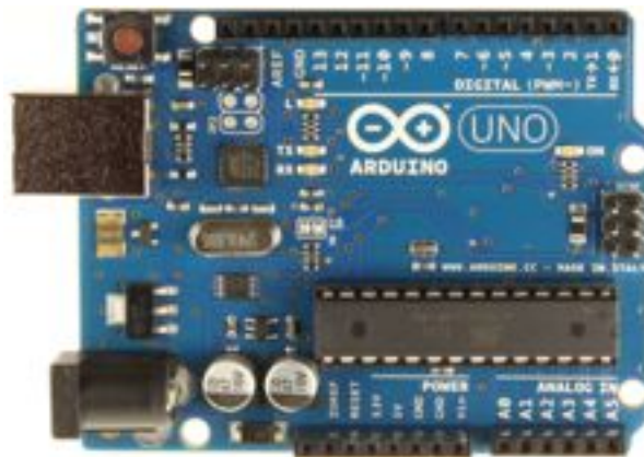
Figure 7: Arduino UNO R3, the control board for the Duck payloads. Image from www.arduino.cc
