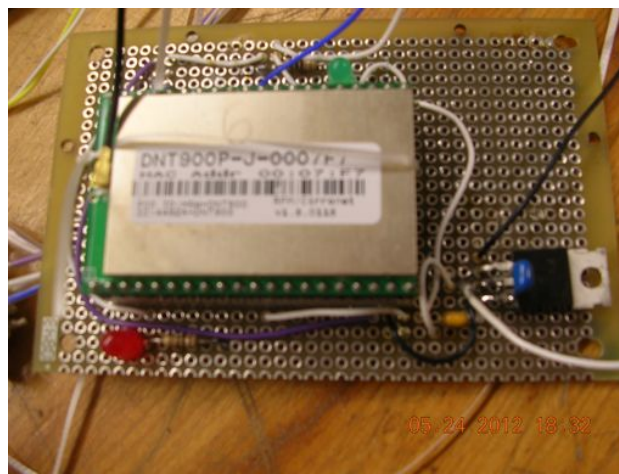
Figure 31: DNT900 radio with support board
